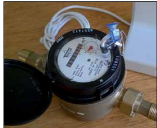
A typical water meter and radio data transmitter. It's what you do with the information and how you interpret it that matters.
