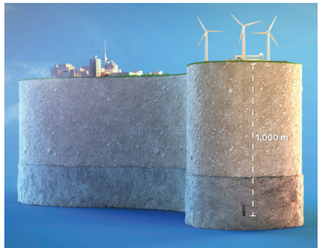
Inside a 250 million year old salt dome below Rüdersdorf, the energy provider EWE is constructing a hydrogen test cavern at a depth of 1,000 m.
